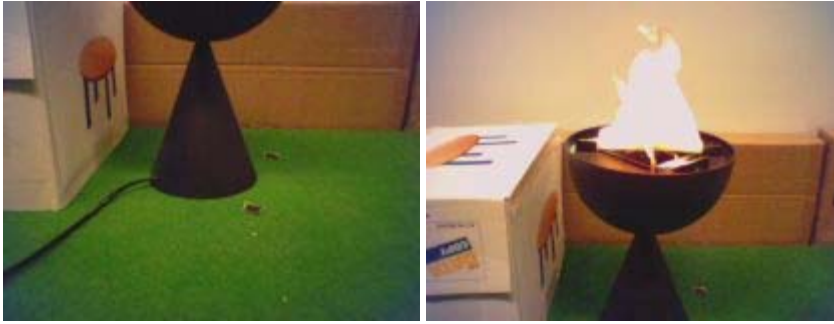
Figure B.1: Pictures of detected fire taken by AIBO. The left picture shows a picture of the fire object made by AIBO during patrolling. The right picture shows the fire object itself.
