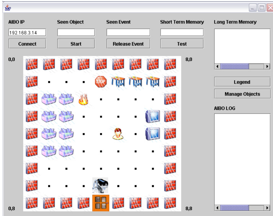
Figure 7.4: Interface of the Main GUI. The picture at the left side is the representation of the simulation of the environment. The other fields will display a certain value so the user can track the patrolling of the AIBO watchdog and know what has happened.
