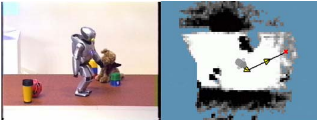
Figure 3.8: Right image shows the occupancy grid and planned path of the left original image.
