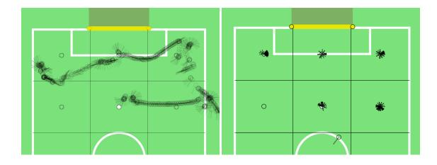
Figure 4: *Left:* The robot walks randomly over the soccer field. Its path according to the already implemented augmented Monte Carlo localization module [3] is depicted as a series of circles and dashes, representing its position and orientation, respectively. *Right:* After walking the random path, the robot has learned to associate certain features with orientations and locations. This is shown as a dash in the corresponding orientation at the center of the location's corresponding grid cell.
