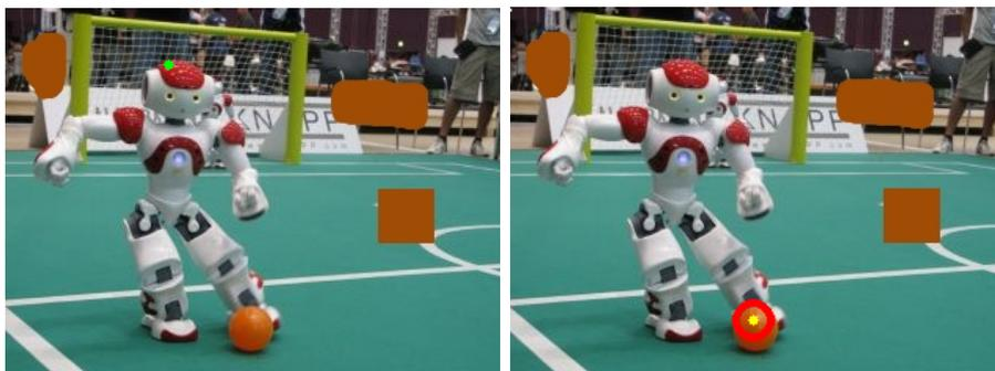
Figure 1: Left: Previous balltracking algorithm, the green dots indicates found ball location. Right: Improved vision module using Hough transform and C++.
